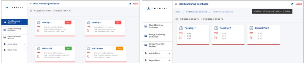
The plant monitoring dashboard provides a consolidated view of all machines at the plant level. It also provides insights into the overall OEE, total power consumption, uptime, current machine state etc.
