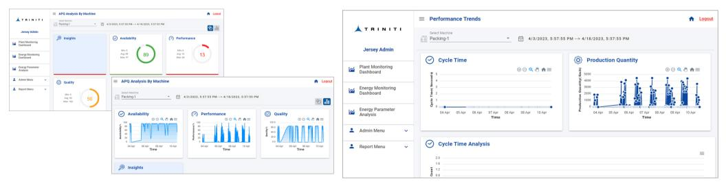
APQ analysis by machine provides details about the calculated Availability, Performance & Quality of machines, generated for OEE for a given period of time The performance trends page displays trends pertaining to total production quantity and cycle time for each equipment, for a selected duration. It will help engineers analyze the machine behavior based on historical trends
