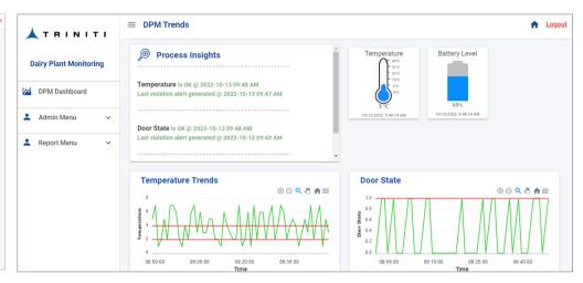
The DPM dashboard provides an integrated view of all chambers & silos. It displays details about the critical events/ parameters like door open/ close, container level, temperature etc.
